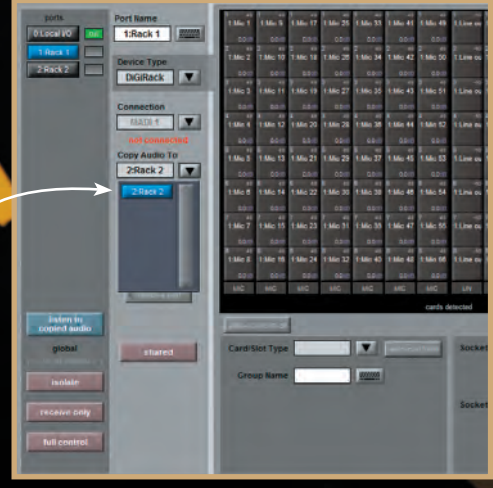
Simple copy to MADI function allowing all remote Mic Pre's to be fed to recording device via console.
