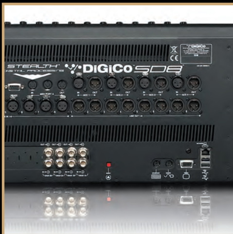
Local I/O 8 Analogue inputs and outputs. 8 AES/EBU (mono).
